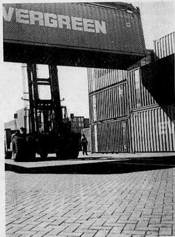
Handling Containers by using Top Loader
