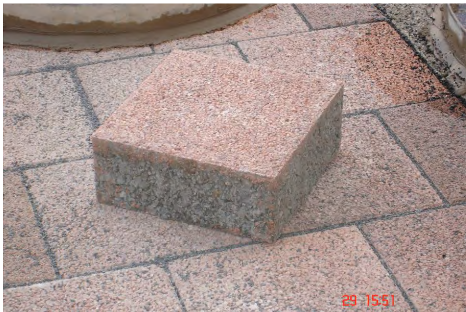
Fig. 3. Example for porous paving block
