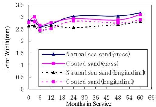
**Figure 8. Changes in joint width**
