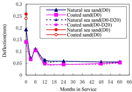
**Figure 3. Changes in deflection (D<sub>0</sub>,D<sub>0</sub>-D<sub>20</sub>)**
