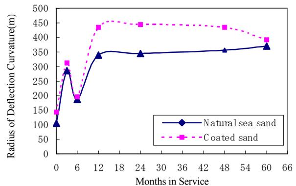
**Figure 4. Changes in radius of deflection curvature**
